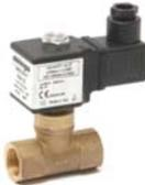
The VMR type valve is a fast opening solenoid valve that is normally closed. When the coil is not energized the spring works on the disc keeping the gas passage closed. When the coil is powered the valve opens. When power is switched off the valve rapidly shuts.
